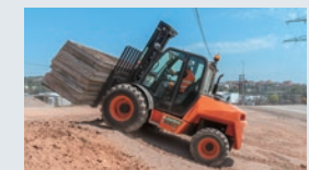
AUSA (Spain) tire-type forklift suitable for traveling on uneven ground
