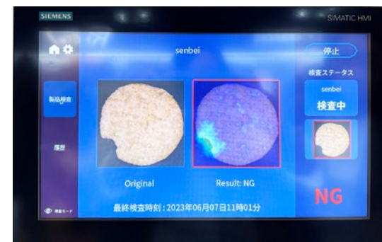
“F[ai]ND OUT EX” visual inspection device
