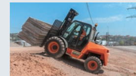
AUSA (Spain) tire-type forklift suitable for traveling on uneven ground
