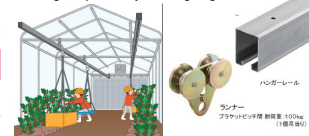
Harvesting transportation system using hanger rails
