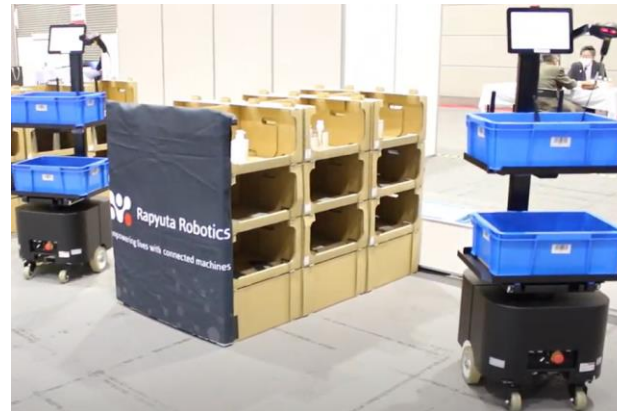
Proposing automation with a Pick Assists AMR for distribution warehouses (Made by Rapyuta Robotics)
